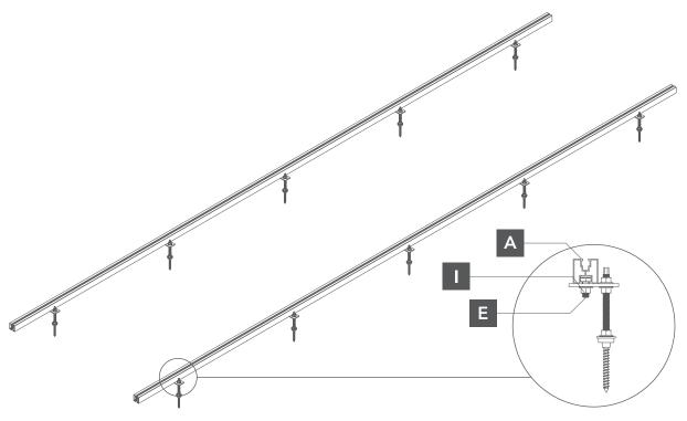
Fig. 6. fastening the mounting rail to the mounting adapter
