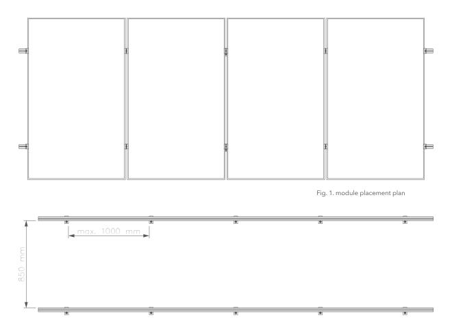
Fig. 2. placement of mounting rails with double threaded screw
