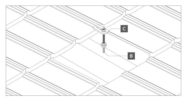
Fig. 4. attachment of the double threaded screw to the roof beams.
