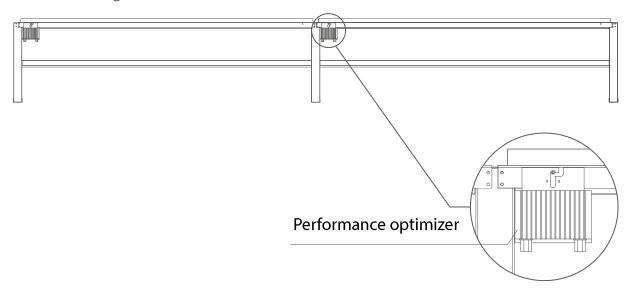
Figure 11. mounting method of the power optimizer.
