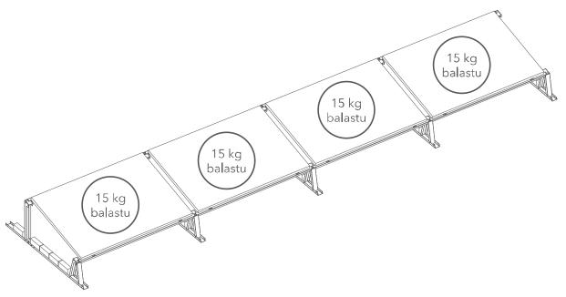
Fig. 6. distribution of the ballast on a row of photovoltaic panels.
