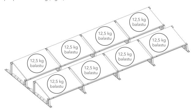
$Fig.\ 7.\ distribution\ of\ the\ ballast\ on\ two\ rows\ of\ photovoltaic\ panels.$
