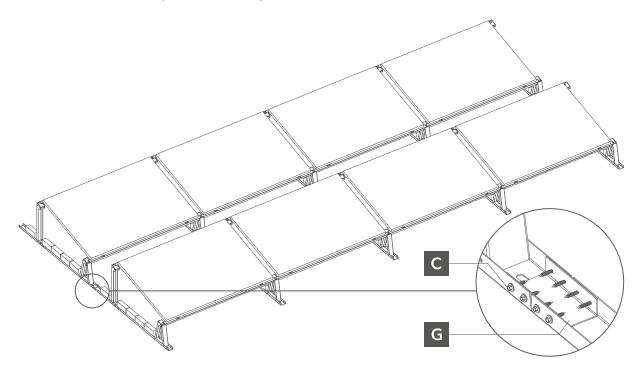
Fig. 5. connecting the mounting triangles with a protractor.
