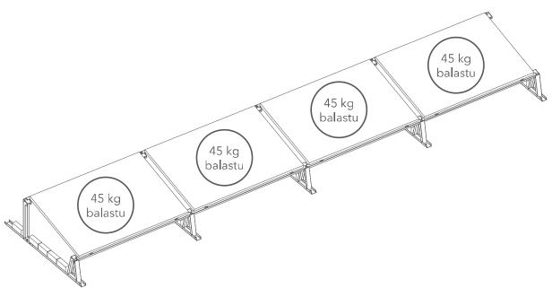
Fig. 8. distribution of the ballast on a row of photovoltaic panels.
