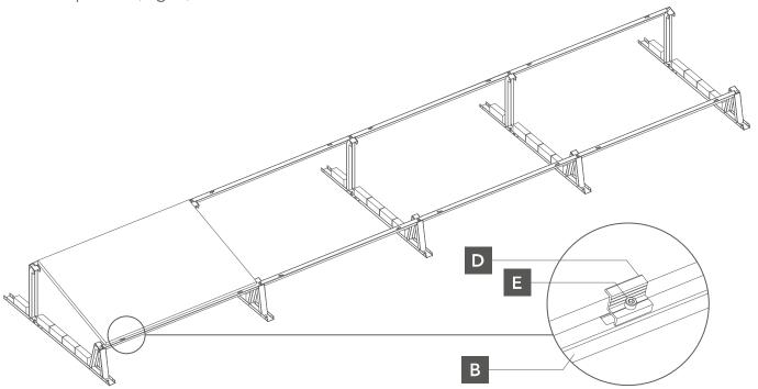
Fig. 4. attachment of the modules to the roof battens
