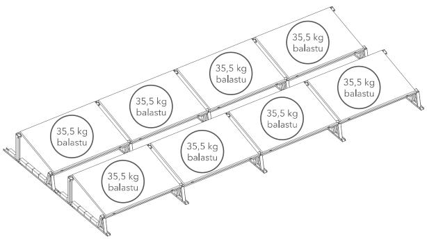
Fig. 9. distribution of the ballast on two rows of photovoltaic panels.
